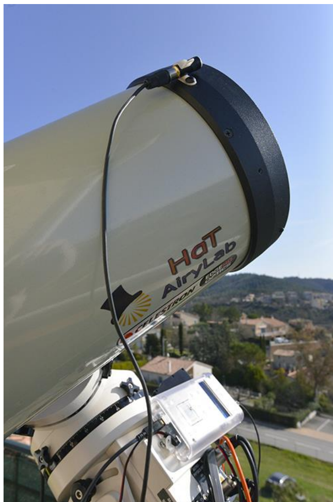
SSM sensor installed on a HaT telescope
