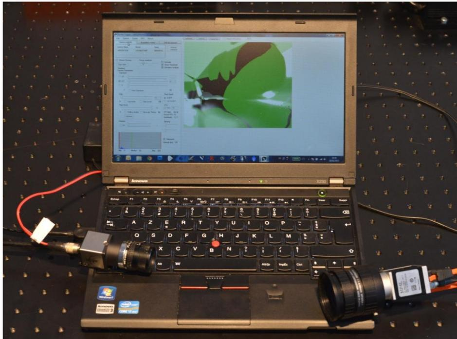
The Genika workstation is an integrated solution for synchronized multi angle image acquisition. Genika Trigger software manages up to three cameras simultaneously on a single laptop to deliver images that are synchronized between each other for further 3D or multi angle analysis.
